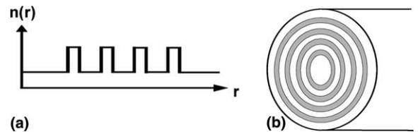
Fig. 1. (a) Refractive index profile. (b) Fiber side view. Shaded regions represent areas of higher-refractive index and unshaded regions represent uniform cladding regions with lower-refractive index.
