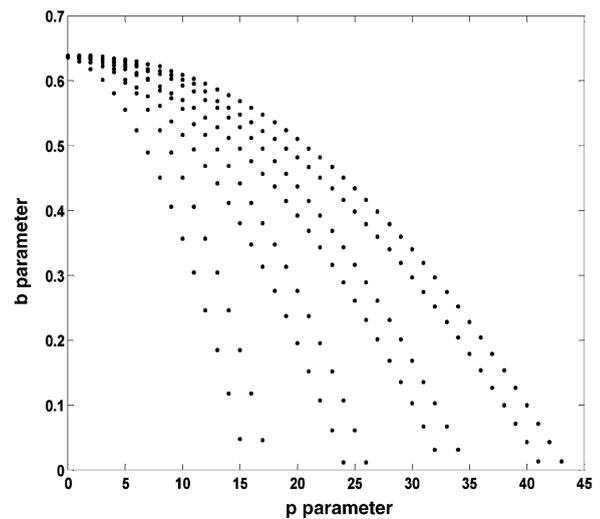
Fig. 2. Numerical simulation results for the  $b$  parameter as a function of the  $p$  parameter. The concentric shell MMF was simulated with shell thickness =  $4\lambda$ , first shell radius =  $25\lambda$ , shell spacing =  $10\lambda$ , and  $V = 3.0807$  from [5].
